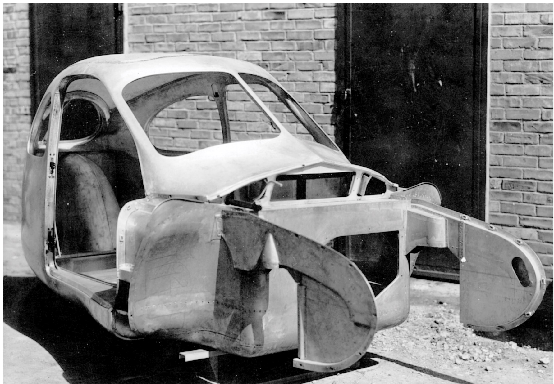
Aluminum Sheet Metal Body Construction (Prototype Model Shown)
