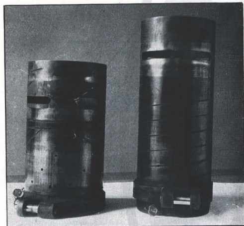
Sleeves 38 h.p. Engine used in R.A.C. test. No wear perceptible.
