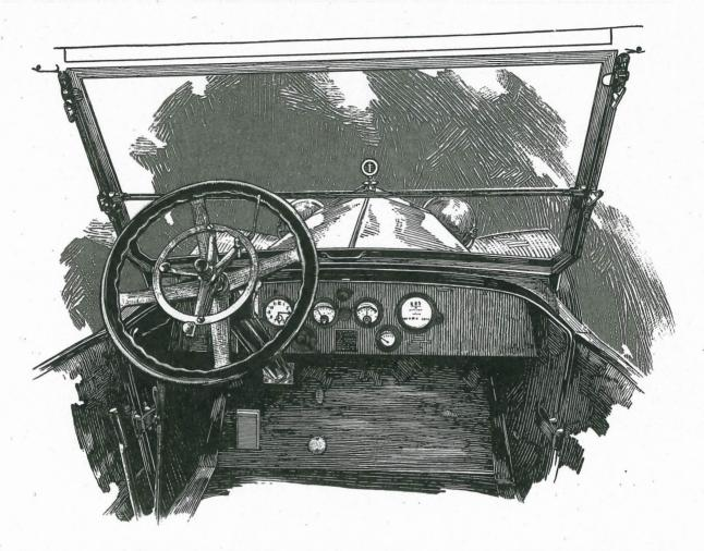
by the car movement and with proper connections made through the controller lever on the steering wheel, the motor becomes a remarkably soft acting electric brake. If more retardation is required, a small foot switch is provided under the toe board of the car, operated by a toe button adjacent to the accelerator pedal, which permits a second step of the electric brake to be applied and resulting in a very powerful electric brake.
