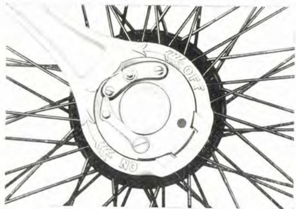
SPANNER IN POSITION FOR REMOVING WHEEL.
