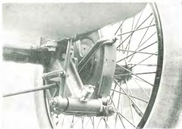
SHOWING ADJUSTMENT AND LUBRICATION OF REAR BRAKES
