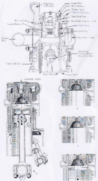
DIAGRAM SHOWING ACTION OF THE DAIMLER SLEEVE VALVES
